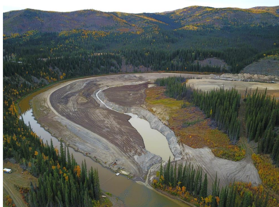
Partially reclaimed placer mine, Yukon. Tailing piles have been flattened, recontoured and top-coated with organic-rich sediments for reclamation
