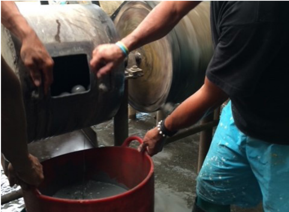
FIGURE 7. A miner using an amalgamation barrel in Colombia
